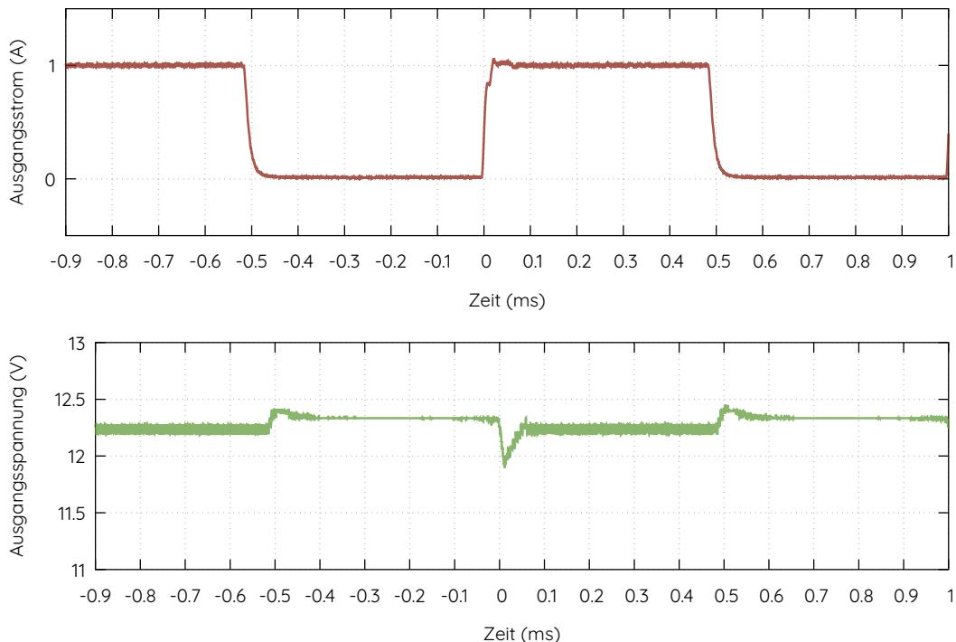
Figure 7: Output voltage behaviour to load current transient
