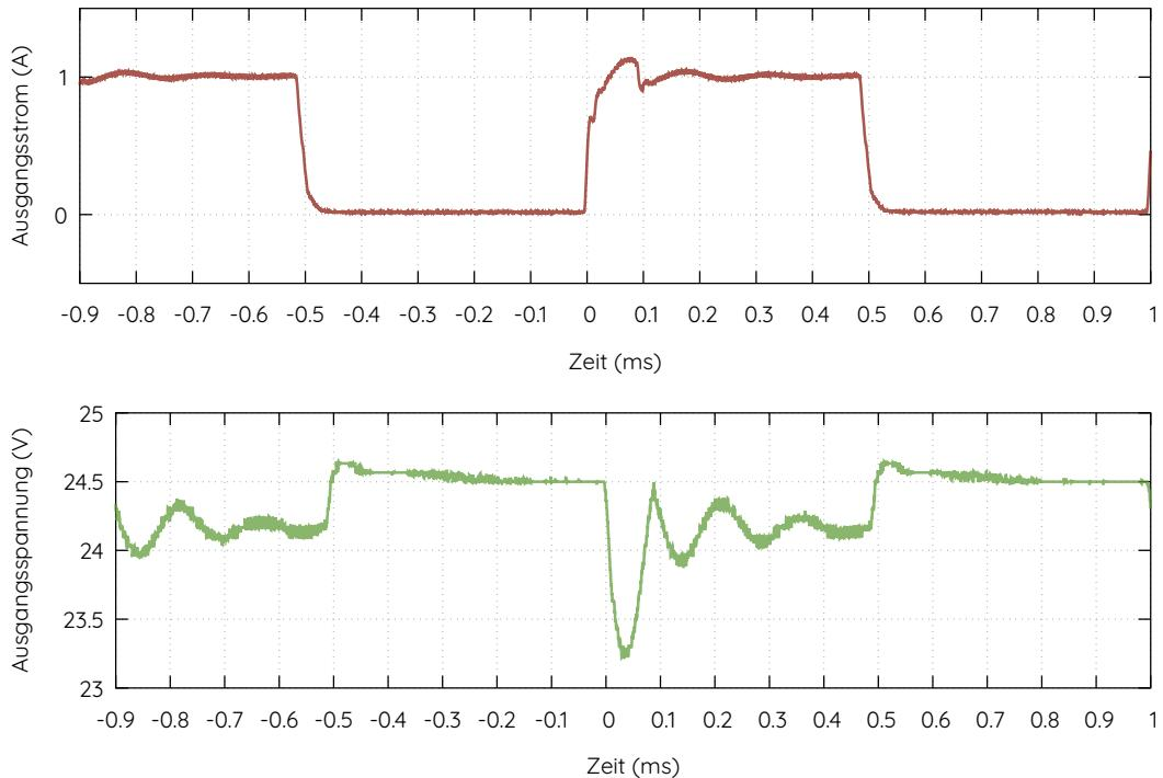
Figure 4: Output voltage behaviour to load current transient
