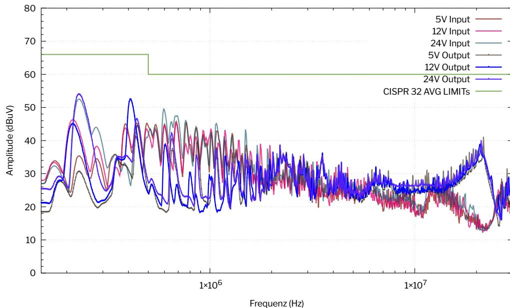
Figure 12: Conducted Output emissions
