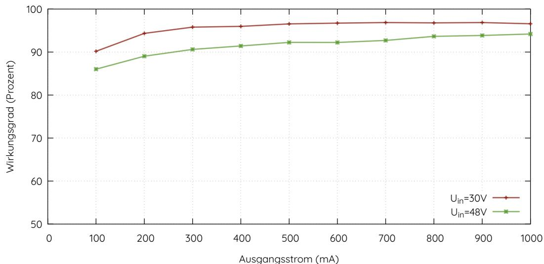
Figure 2: Efficiency of the 24V Variant over Output Current
