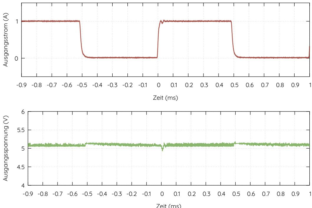
Figure 10: Output voltage behaviour to load current transient
